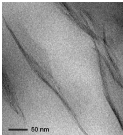
Figure 1 High-resolution transmission electron micrograph showing single platelet layers. 1
